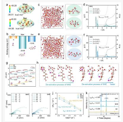
Solvation structures and their impact on desolvation/deposition dynamics in three electrolyte formulations.
