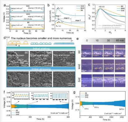
Comparative analysis of zinc deposition/stripping behaviors and electrochemical properties in three electrolyte formulations.
