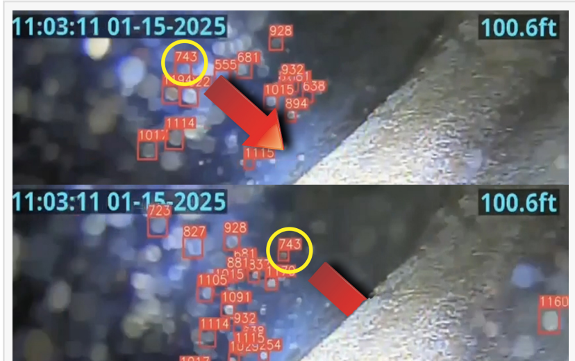
Electro Scan's AI traces individual water particles to confirm leak locations, by clock position.
