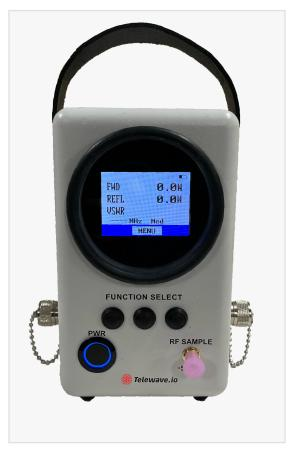
Unlike traditional wattmeters, the 44D-LX requires no field calibration, frequency elements (slugs), or correction tables across its specified temperature or frequency range.
