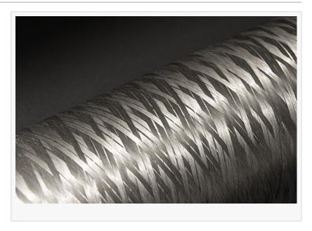
fiber. This new fiber, AluCoat, was developed by FibreCoat to address the need for lightweight, conductive materials in applications such as electromagnetic interference (EMI) and radio-frequency interference (RFI) shielding, as well as thermal management for electric vehicles, consumer electronics, and energy storage.
