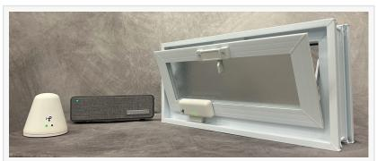
To demo its Smart Home Sensor Technology at CES, Powercast developed two sensors – water detection (far left) and window position – that are powered over the air by an RF transmitter. One transmitter can power all sensors installed up to 25 ft. away.
