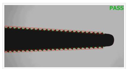
The Tooth Checker™ tool can check that either crests, roots, or both, are in tolerance, such as on this medical rasp
