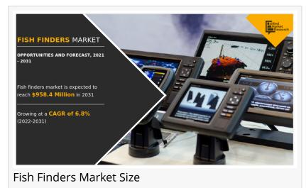
purposes. A fish finder helps the user to detect a fish school and provides the user with different underwater information, such as water depth, distribution of fish school, and the condition of the seabed by transmitting ultrasonic waves into the sea and receiving its reflection back to the receiving circuit on the boat.
