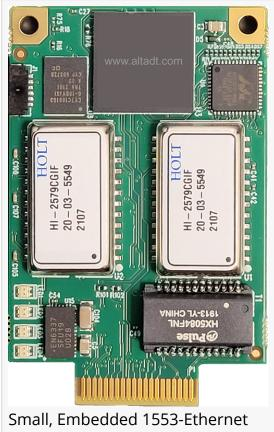
Small, Embedded 1553-Ethernet Converter Mezzanine
