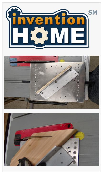
complexity, including rip cutting jigs, crosscut jigs, miter jigs, and box jigs. These jigs are tools designed to help woodworkers achieve precise, repeatable cuts, often improving the accuracy and ease of making straight or angled cuts.
