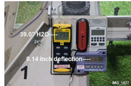
11. Target pressure of 38.8PSI achieved with 0.14-inch of deflection in the system.
