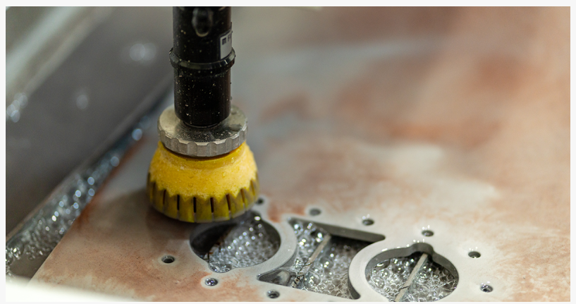
Specialist Waterjet Cutting Head Processing Stainless Steel
