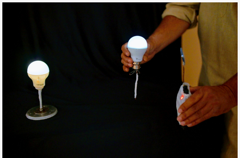
The INFRGY system of transferring electricity via radio frequency
