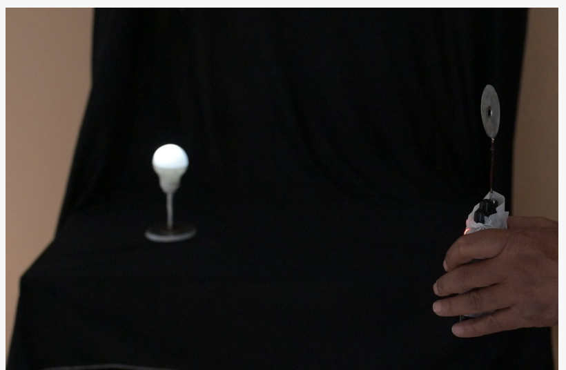
Transmitter and bulb with circuitry to receive and convert RF signals to electricity
