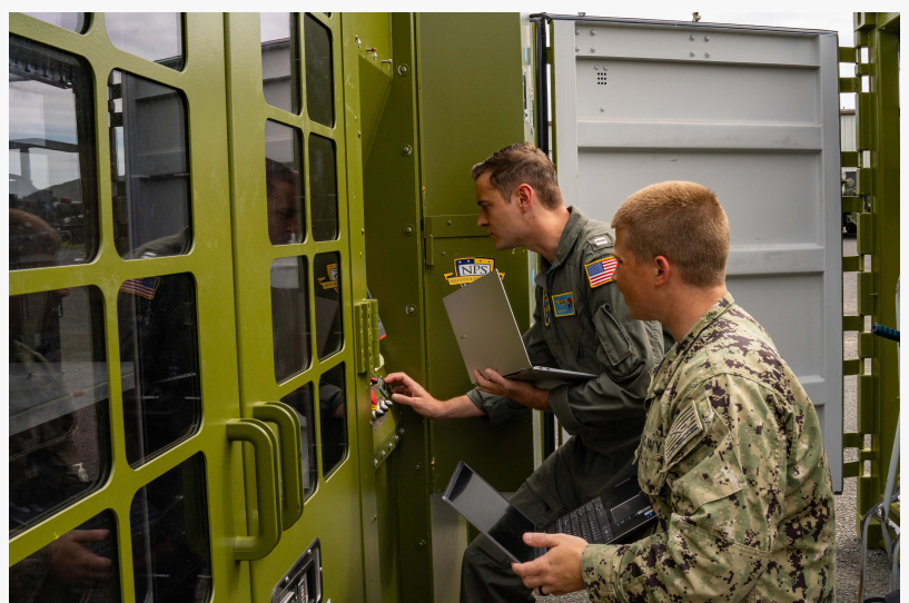
U.S. Navy Lt. Andrew Staley and Lt. Daniel Lukac, students at the Naval Postgraduate School (NPS), prepare the printing of a ship part using an XSPEE3D expeditionary cold spray printer at Marine Corps Base Hawaii during Exercise Trident Warrior 2024.
