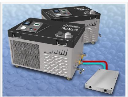
The Industrial Cooling Distribution Module (iCDM) from ATS is a plug and play system that houses all components of a liquid cooling loop in one portable enclosure and connects to cold plates and other liquid cooling devices for electronics.
