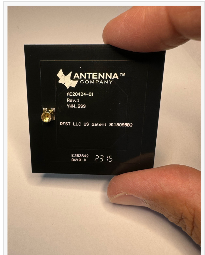
The AC20424-01 (RF Coupler) resides inside the smart meter
