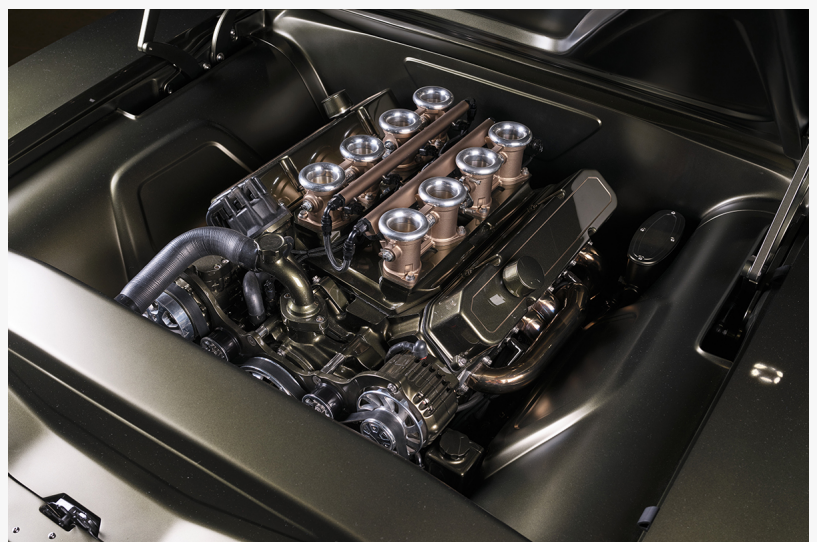
The original 440c.i. engine has been highly modified.
