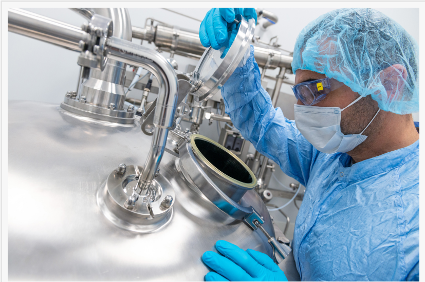
An operator trained in GMP conditions and wearing the recommended equipment, is checking the inside of the fermenter tank
