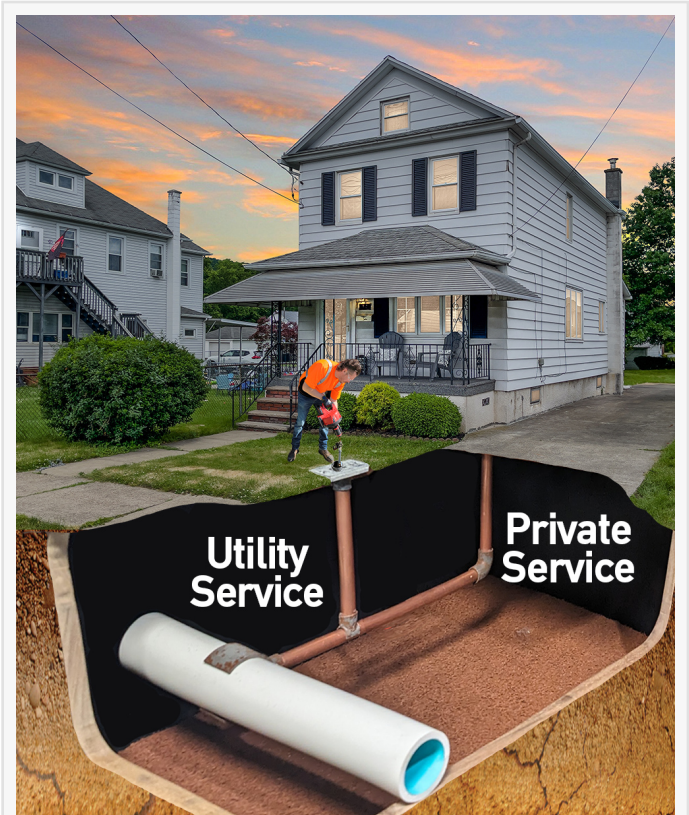
The USEPA requires all 50,000 drinking water system providers to inventory both utility owned services, typically from water main to meter, and private property owned water services and private services.
