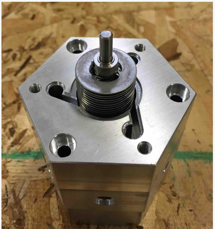
Revolutionizing Fluid Dynamics: This Modular Block features stacked discs designed for non-cavitation fluid pumping, drawing inspiration from Tesla's groundbreaking original invention to efficiently pump or expand fluids without loss of performance or integrity.
