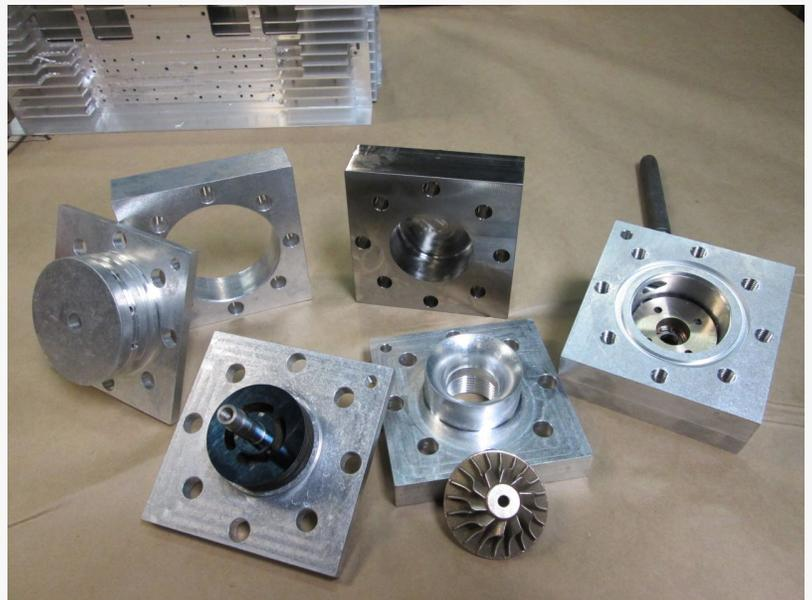
Modular blocks for processing and sampling of gases and liquids, and more specifically to devices allowing rapid construction of fluid reactors, distillers, extractors, homogenizers, filtration/separation devices, and process models.
