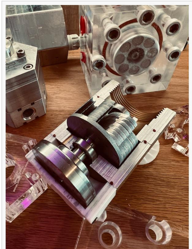
Modular Blocks with Magnetic Couplings: A Revolutionary Way to Safely Separate Pressurized and Non-Pressurized Gases and Fluids for Pumping and Expander Applications.
