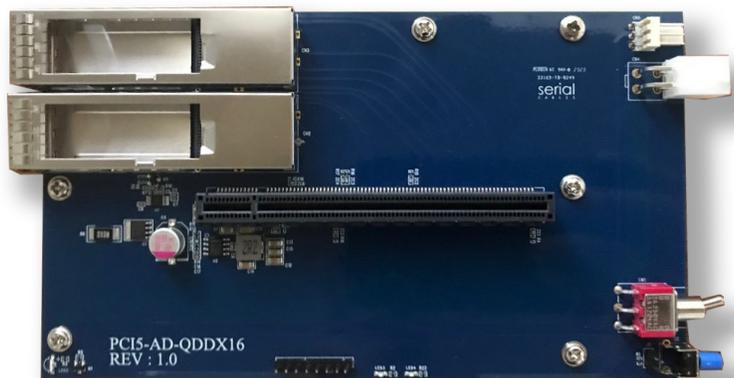
Gen5 PCIe/CXL QSFP-DD - x16 AIC adapter board
