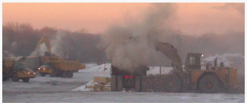
Pulverizing demolition waste creates fine particles which cause huge clouds of toxic dust at the Lordstown Landfill. The dust can include asbestos, lead paint, silica, mold and fiberglass. It also provides an enormous feedstock for poison gas-producing bacteria
