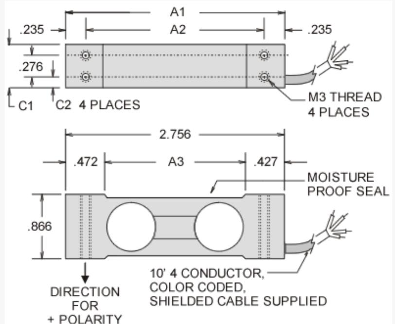
LSP Series Beam Load Cell Specifications
