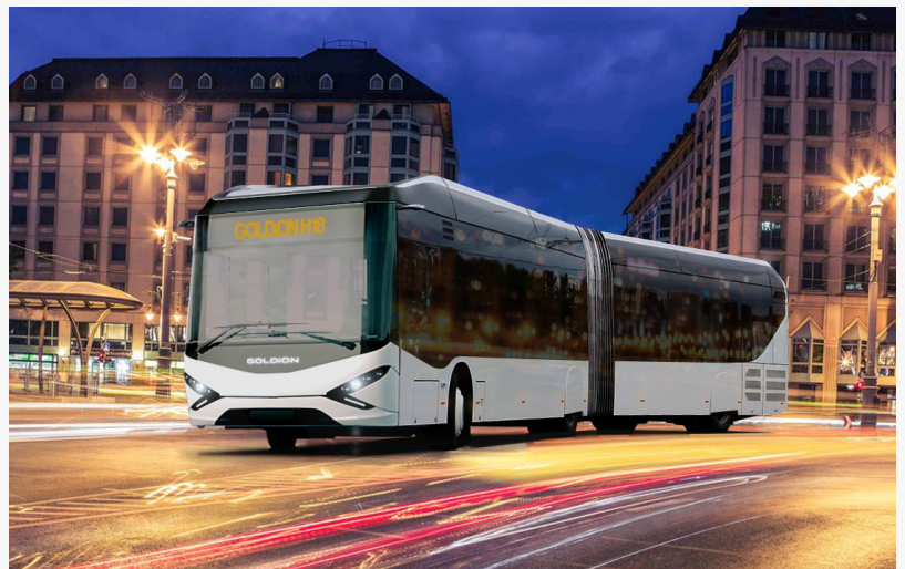
GOLDiON H18: A Special Plug-in Hybrid with Battery & Fuel Cell Drive Articulated Bus
