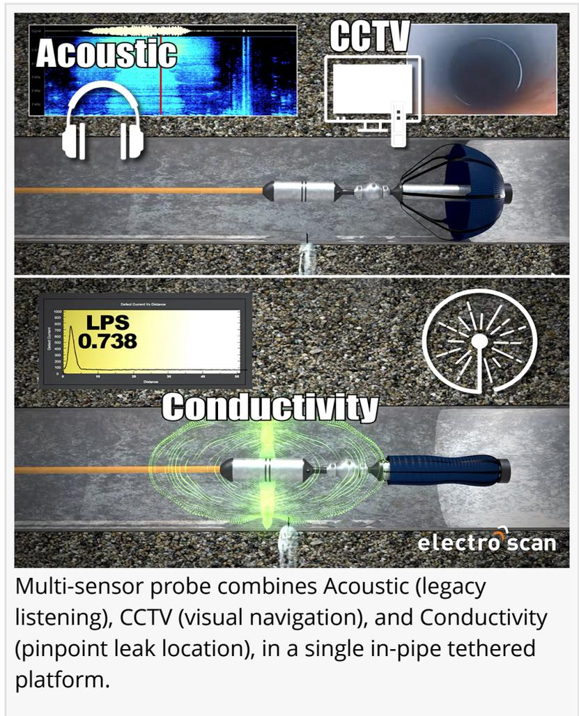
The combination with Electro Scan's electric current-based sensor and high-definition camera allows framework contractors and water utilities to locate and quantify all leaks immediately following each survey and before leaving the project location.
