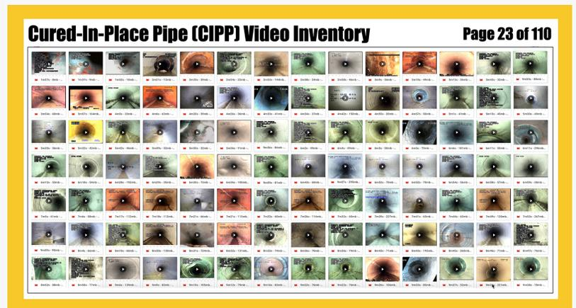
Hansen Analytics maintains one of the largest video libraries of Cured-In-Place Pipe (CIPP) defects to help teach machine learning algorithms to identify and label anomalies to be followed up with low voltage conductivity leak detection.
